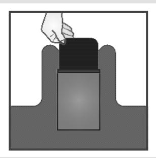
The directionality and orientation of CARNA™ SA inserts have no impact on performance. Each CARNA™ SA insert is cut uniquely for the back and front soft armour ballistic inserts.
