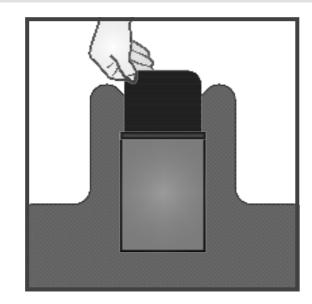
The directionality and orientation of CARNA™ SA inserts have no impact on performance. Each CARNA™ SA insert is cut uniquely for the back and front soft armour ballistic inserts.
