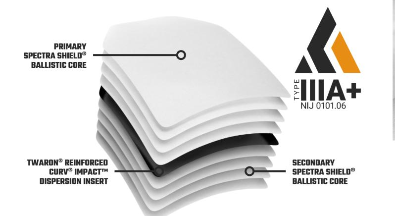
Forgoing flexibility on behalf of its highly specialised purpose, the layup has been specifically engineered to mitigate the post-impact trauma and fragmentation threats that can occur behind ICW (in conjunction with) hard-armour systems.
